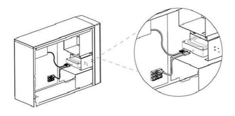
Put MRA263 into 3.5" HDD slot position, fix two screws on each side, four screws in total.
