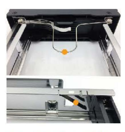
Add low cost of metal components to support thinner HDD in vertical PC environment.
