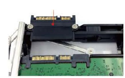
Non-scratch SATA connector (NSS) allows Hard Drive hot-swap life cycle for more than 50,000 duty cycles.
