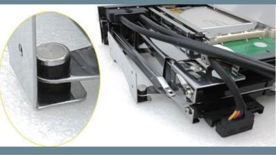
4 anti-vibration silicone rubbers on two sides of products to absorb the vibration from moving and resonance
